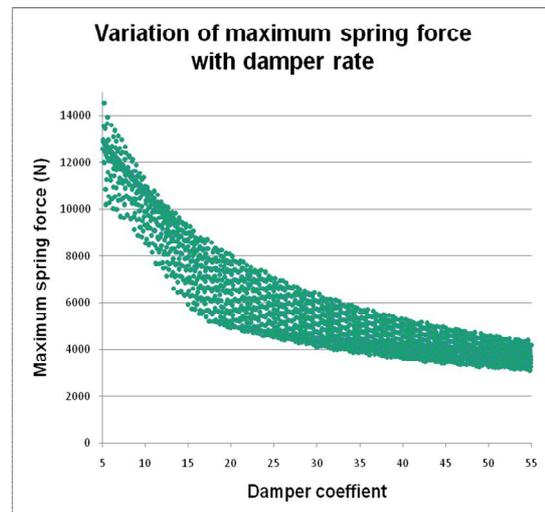
The Engineer can begin to understand the distribution of the spring force population and how the performance of the damper affects the maximum spring force.
