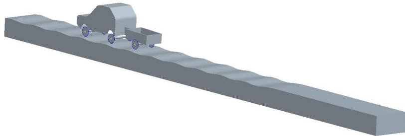
During the motion, the forces experienced by the spring and the damper were recorded and for a fixed road surface profile, the trailer variables were modified.
