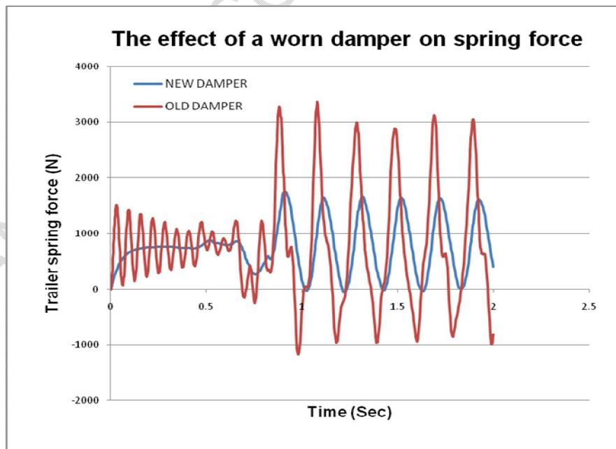
The initial oscillations of the trailer for a worn damper are in fact damped out by the suspension of the towing vehicle. This view is of design input extremes.
